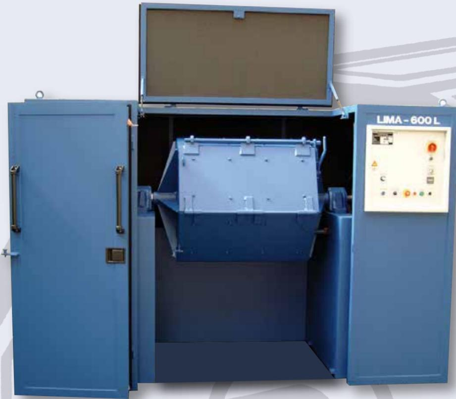
The doors can be opened to the extent that also loading from top by means of a tip container or a hoist can be performed. The aid of touch control, the drum can be moved into any position.
