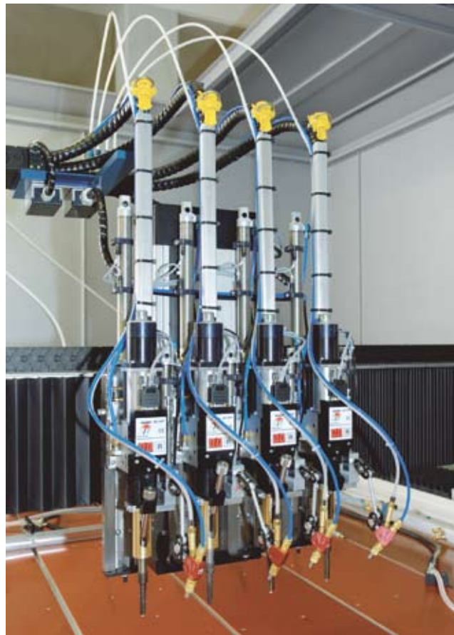
Four SK-5AP welding heads with digital display for precisely measuring the lift-off distance and the immersion depth
